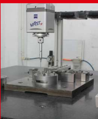
ZEISS三坐标测量仪检测 ITS卡盘 ZEISS coordinate measuring machine detects ITS Chuck
